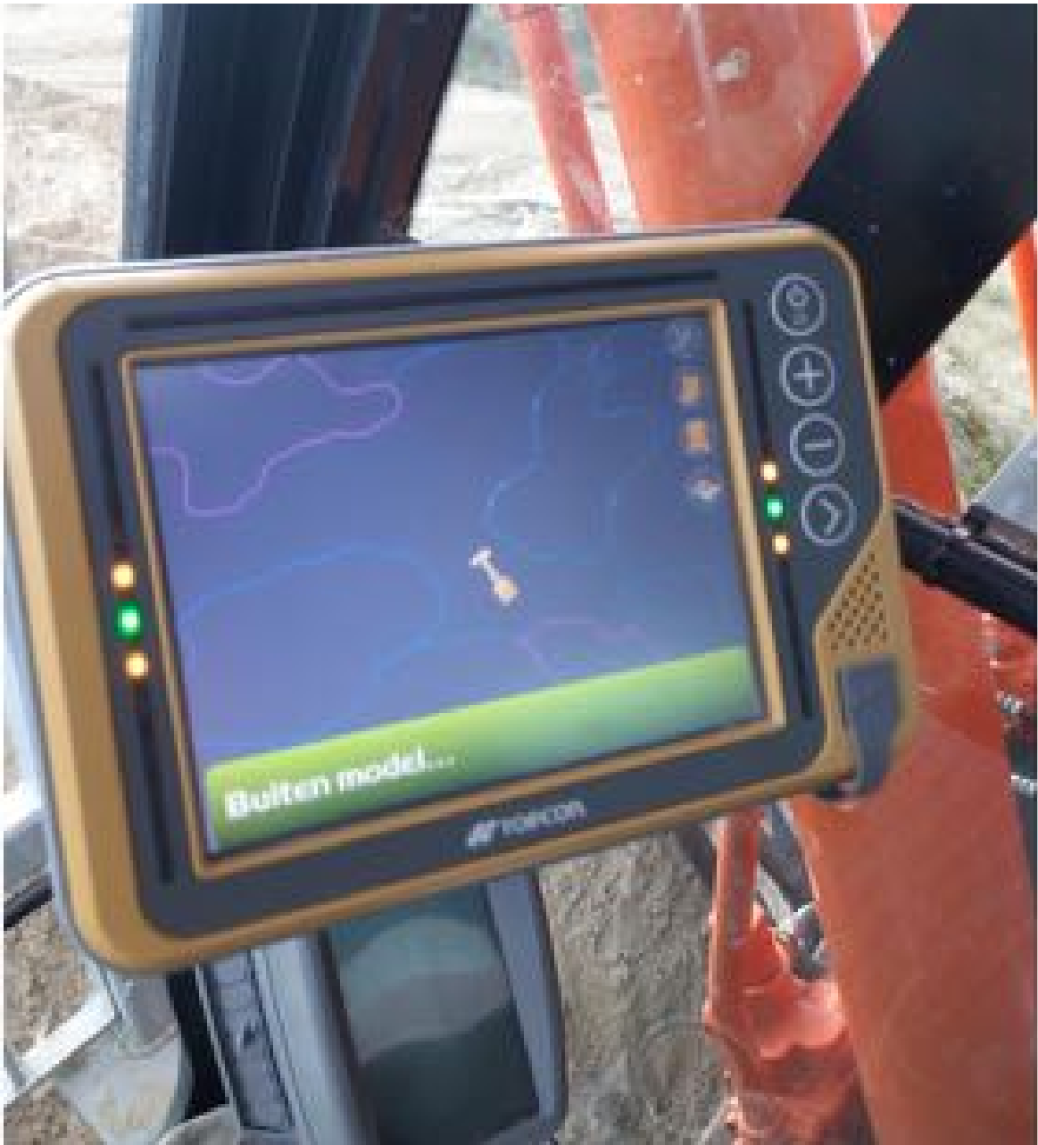
Figure 20: A GPS was used in the excavator in order to excavate the vegetation according to the depths specified in the best practices study ( © Reinhardt Strubbe).
